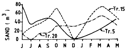
Fig. 7—Volume of sand per metre length of the beach
