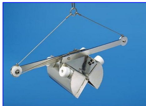
Long arm, warp rigged Van Veen grab in sampling operation. (Redrawn from Rumohr 1999.)
