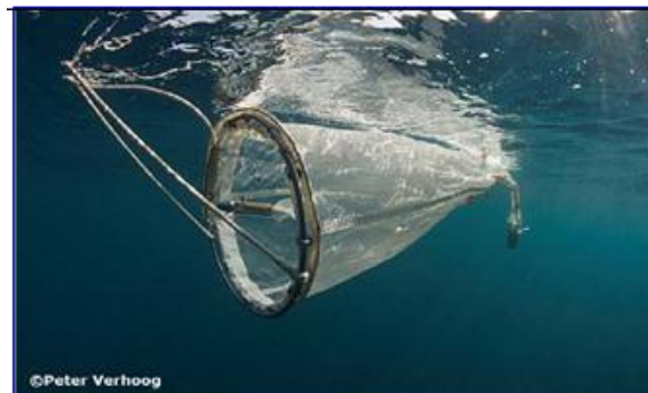
Sampling with flow meter
